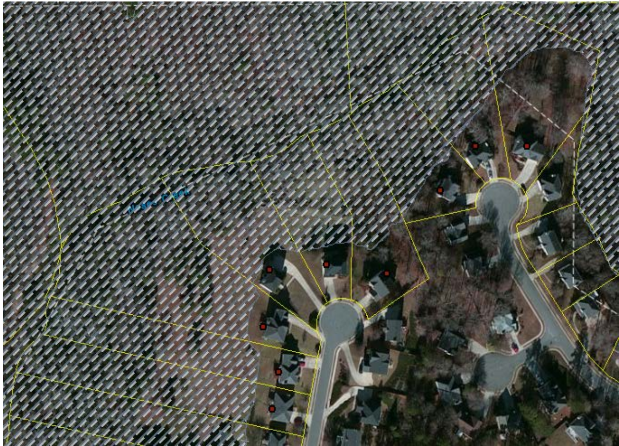
Figure 1: Example of study area floodplain. Hashed grey area represents extent of 500-year floodplain. Red dots represent the point at which ground elevation was measured.
